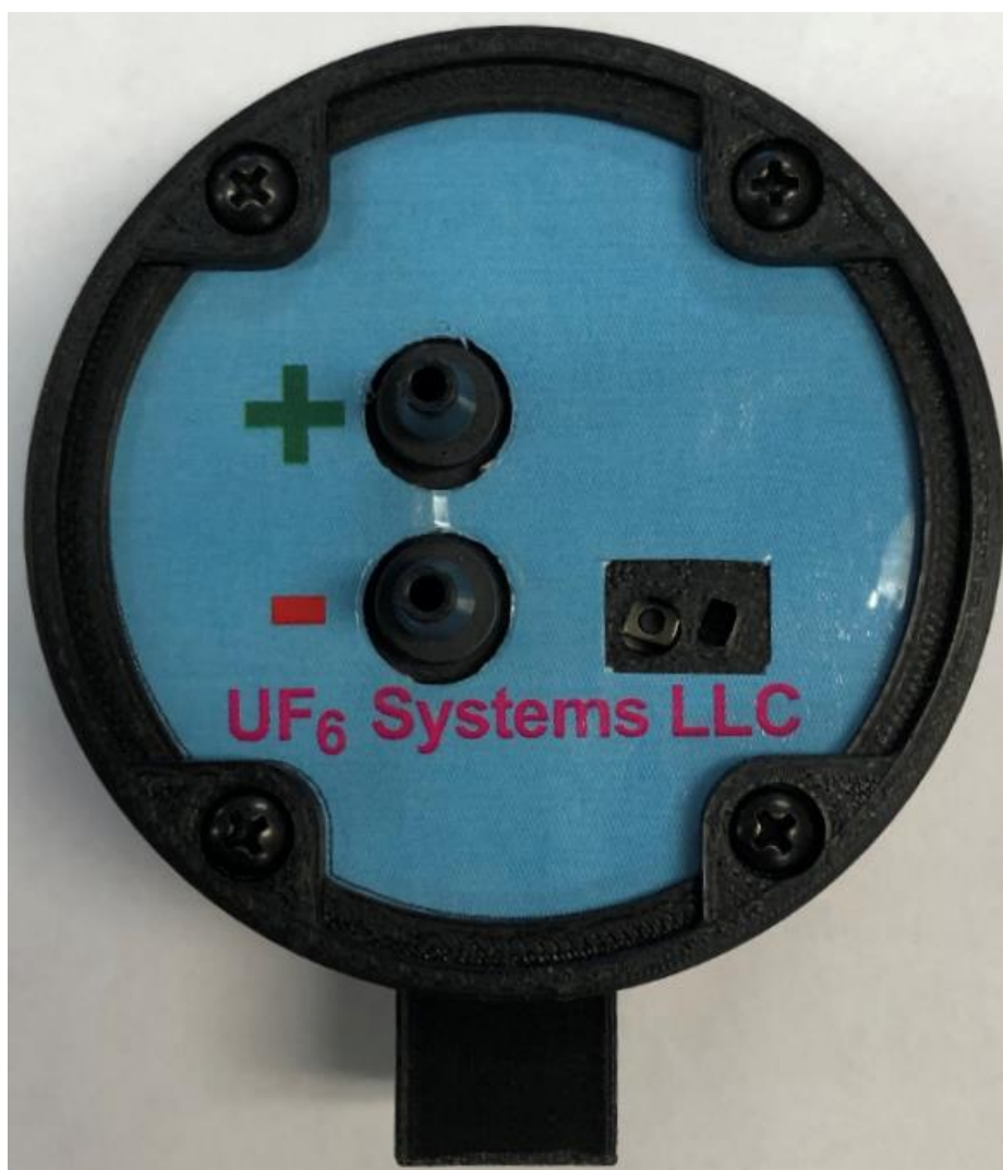
Rear View showing pressure ports
