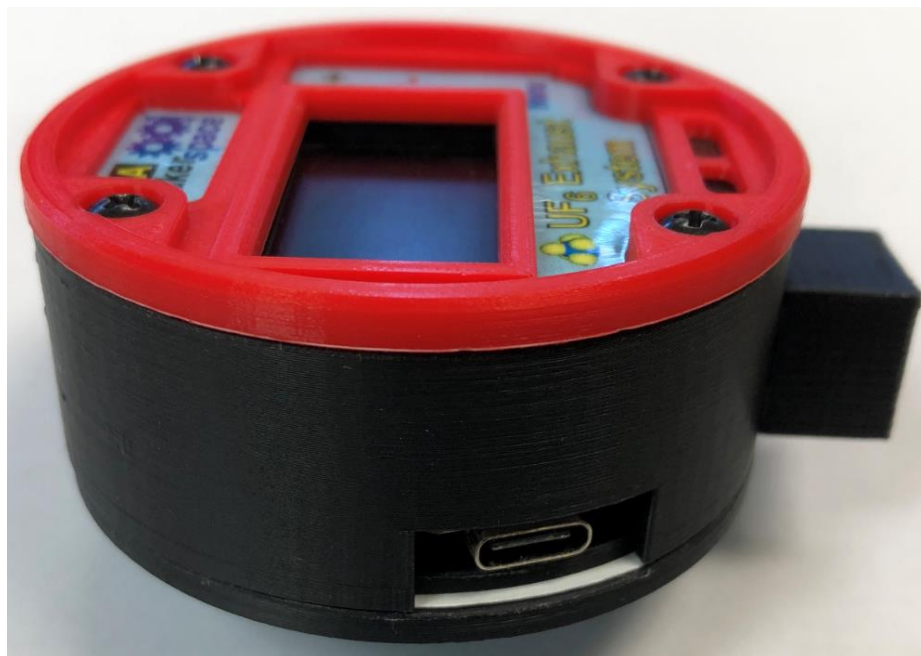
Side View showing USB-C connector for power and programming
