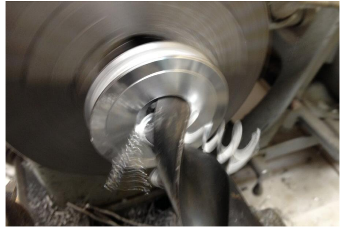
Using a boring bar to chamfer edge
