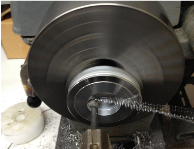
Using a boring bar to finish bore size
