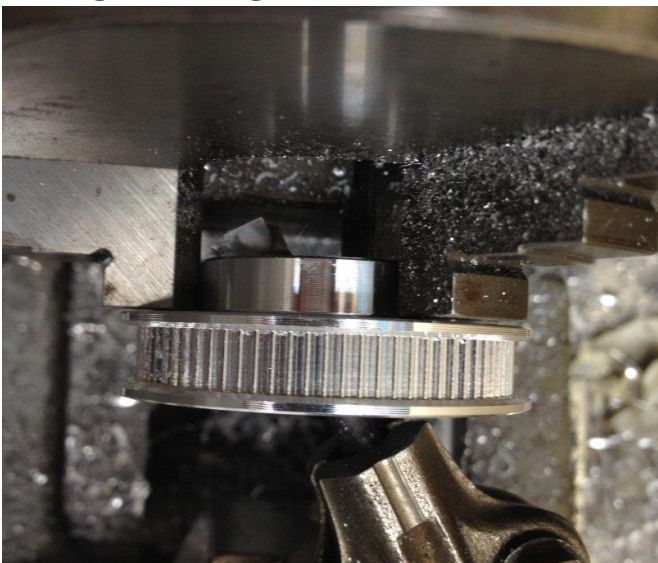
Using a boring bar to chamfer far edge
