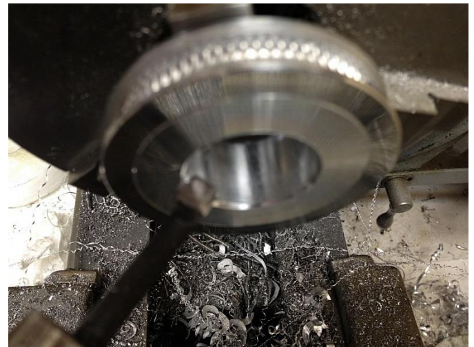
Using a boring bar to chamfer edge
