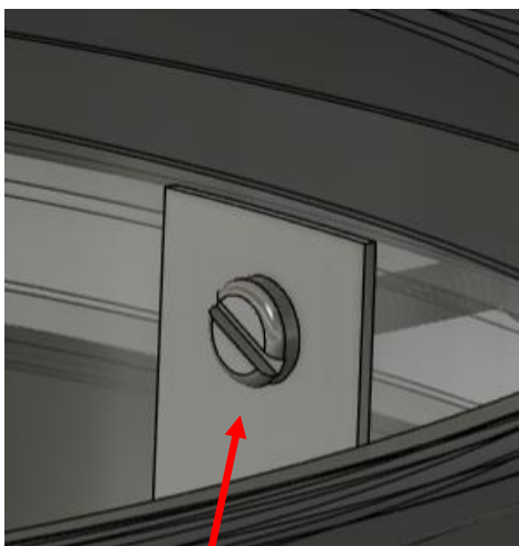
Lead sheet tab with screw (Titanium or Nylon)
